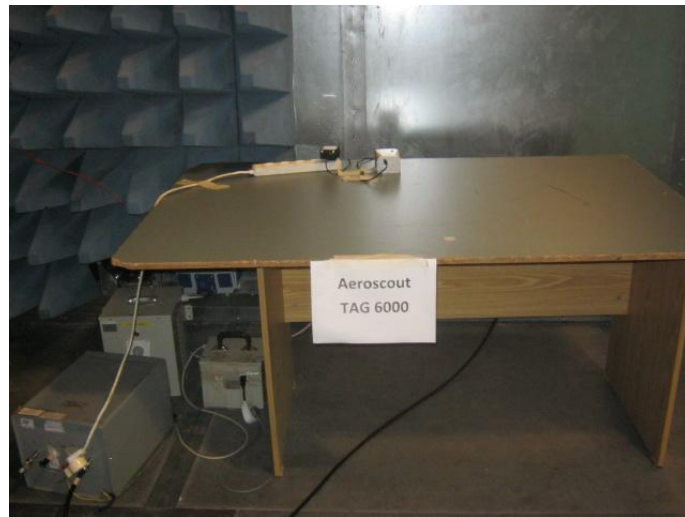
Figure 3. Conducted Emission From AC Mains Test
