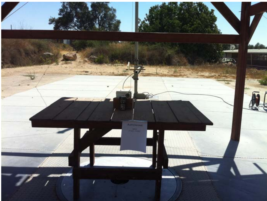
Figure 3. Radiated Emission Above 1 GHz Test
