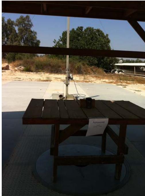
Figure 2. Radiated Emission Below 1 GHz Test
