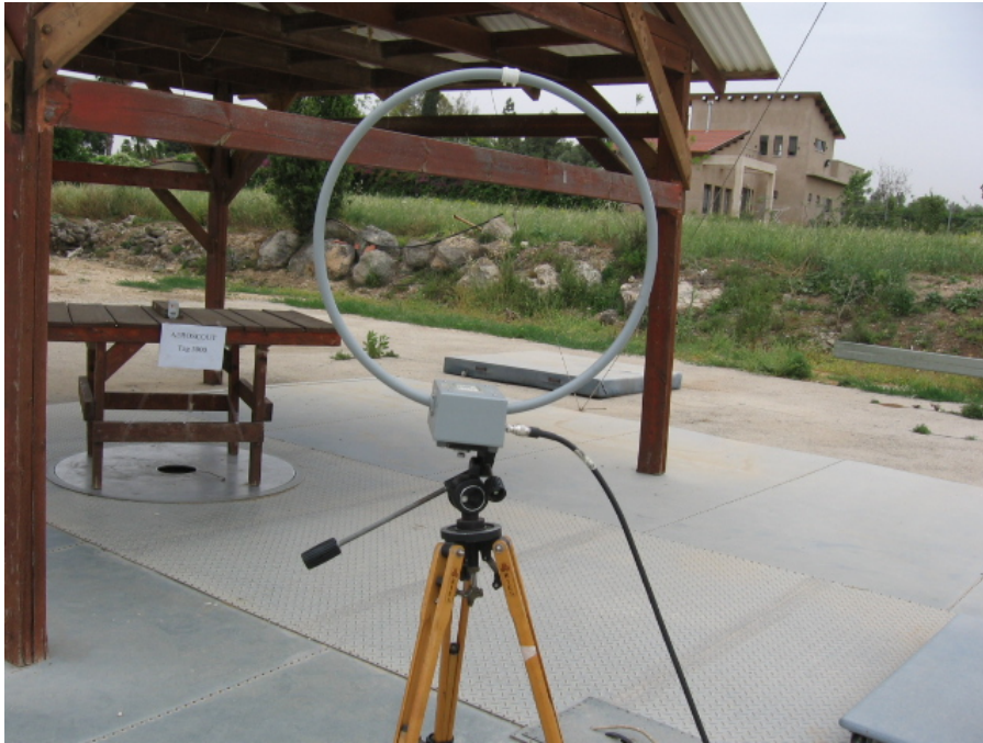
Figure 3. Radiated Emission Test
