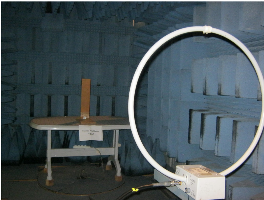
Radiated Emission Test, 0.009 – 30MHz
