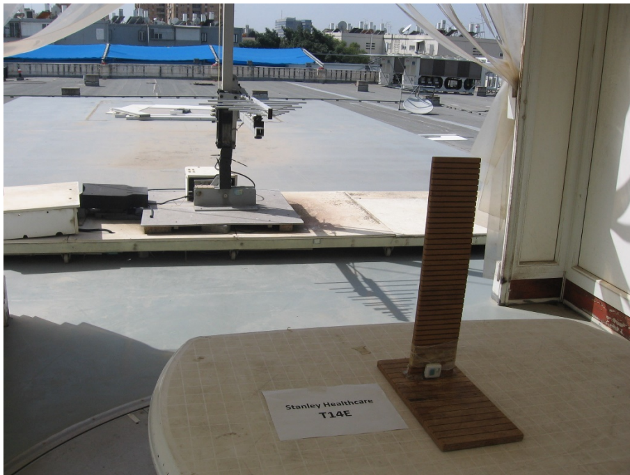
Radiated Emission Test, 200-1000MHz
