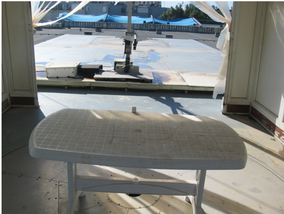
Radiated Emission Test, 200-1000MHz
