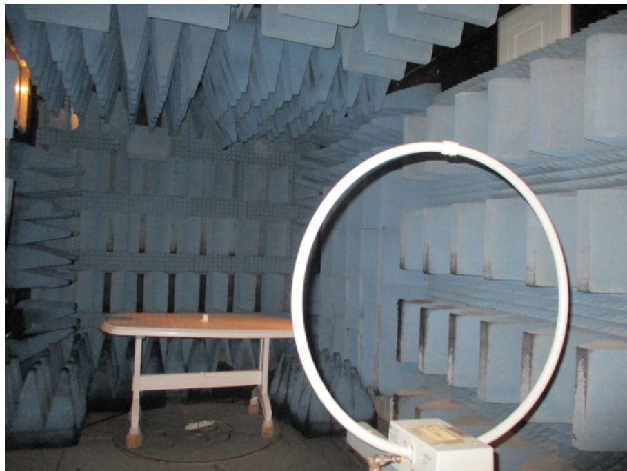
Radiated Emission Test, 0.009-30MHz
