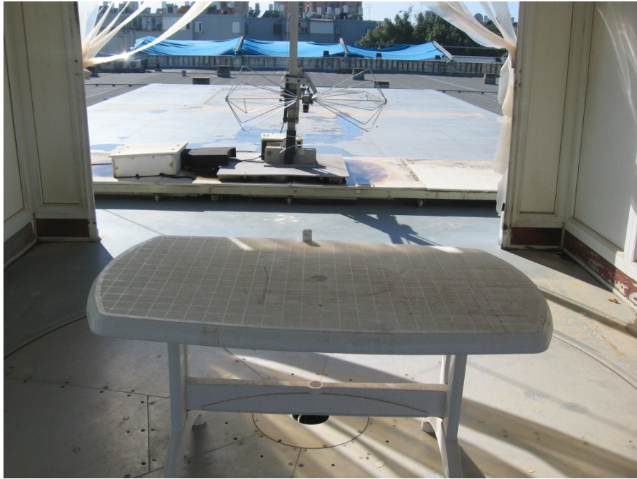
Radiated Emission Test, 30-200MHz
