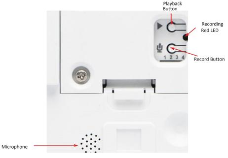
The Playback and Record buttons are found on the back of the monitor. The microphone is located outside the battery compartment as shown above.
