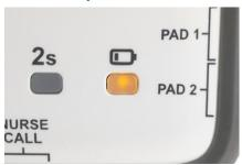
The Low Battery reminder (LED and audible message) initiates approximately 7 days before the battery is fully drained of power. It is important to replace all three batteries at the same time.
