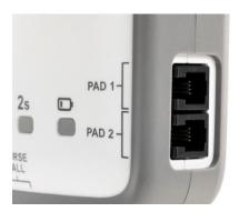
Sensormat Pad (PAD 1 and PAD 2) - These are used to connect two pads at the same time. See "Using Sensormat Pads" on page 17.
