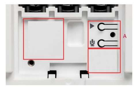
A. The Playback and Record buttons, Recording red LED and the Microphone are used to record custom audible/voice messages up to a maximum of 15 seconds, after which a Positive Confirmation Tone sounds. For instructions on recording a custom message for an Exit Alarm, see "Recording Custom Pad Alarms" on page 14.
