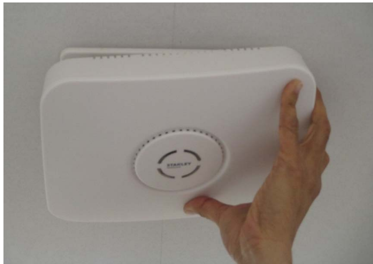
Figure 17: Attaching the Controller to the Mounting Adapter
