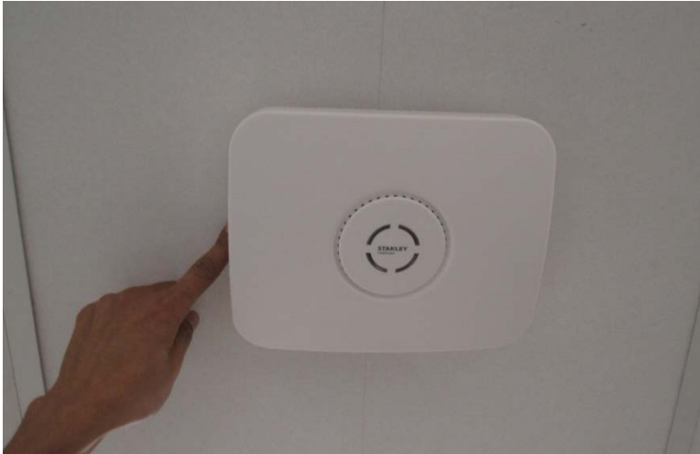
Figure 18: Releasing the Controller from the Mounting Adapter
