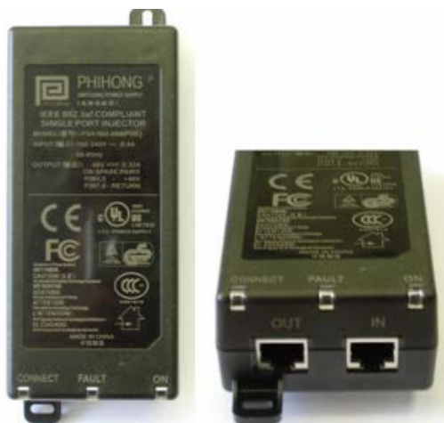
Figure 6: 110/220 VAC to 48VDC PoE Single-Port Injector
