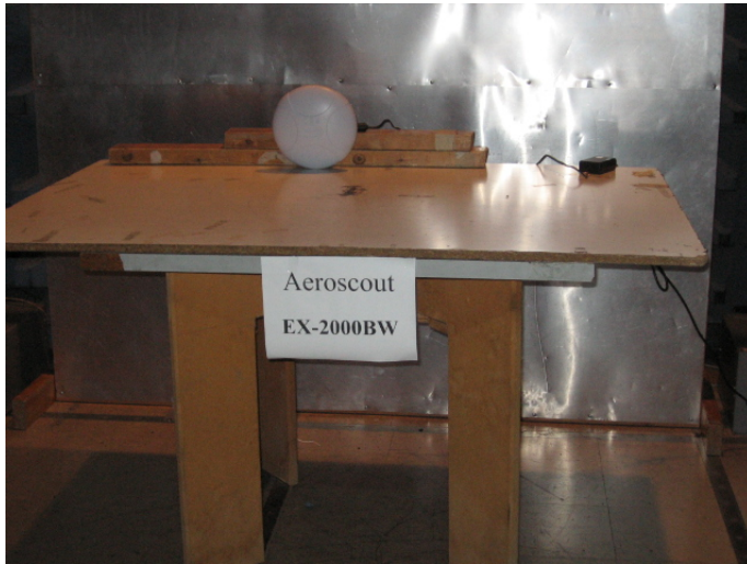
Conducted Emission From AC Mains Test Set-up
