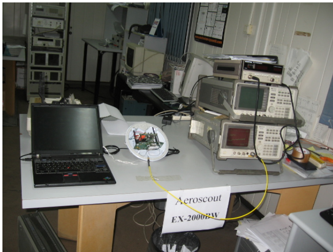
Conducted Antenna Port Tests Set-up
