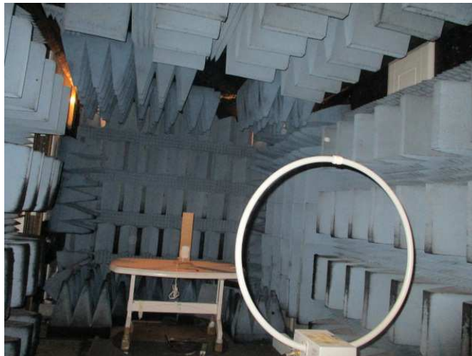
Figure 2. Radiated Emission Test, 0.009 30.0MHz
