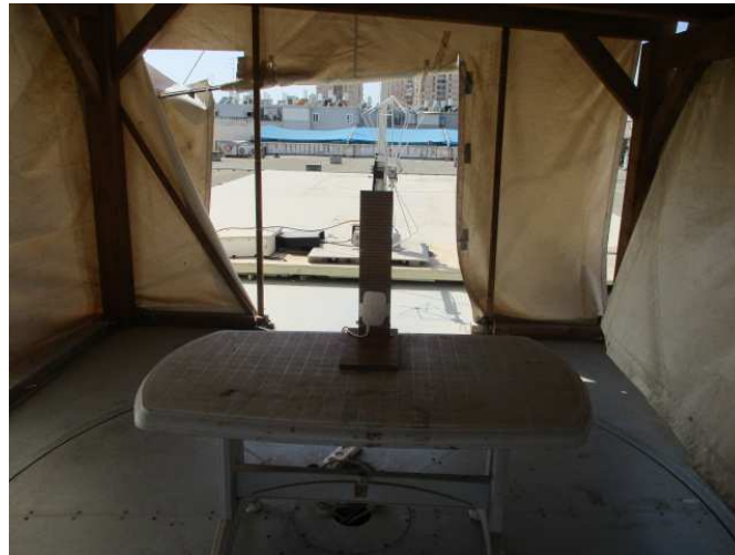
Figure 3. Radiated Emission Test, 30.0-200.0MHz
