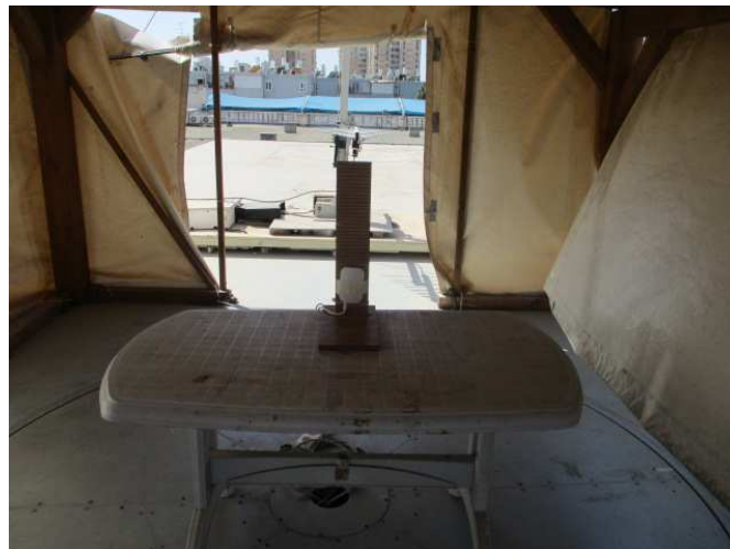
Figure 4. Radiated Emission Test, 200.0-1000.0MHz
