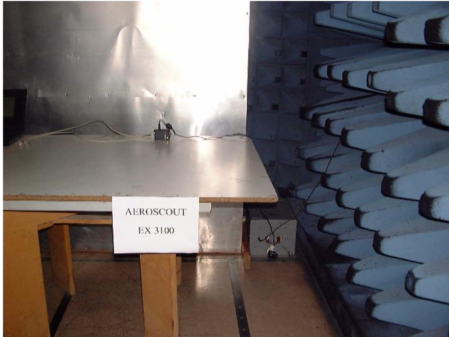
Figure 1. Conducted Emission Test.
