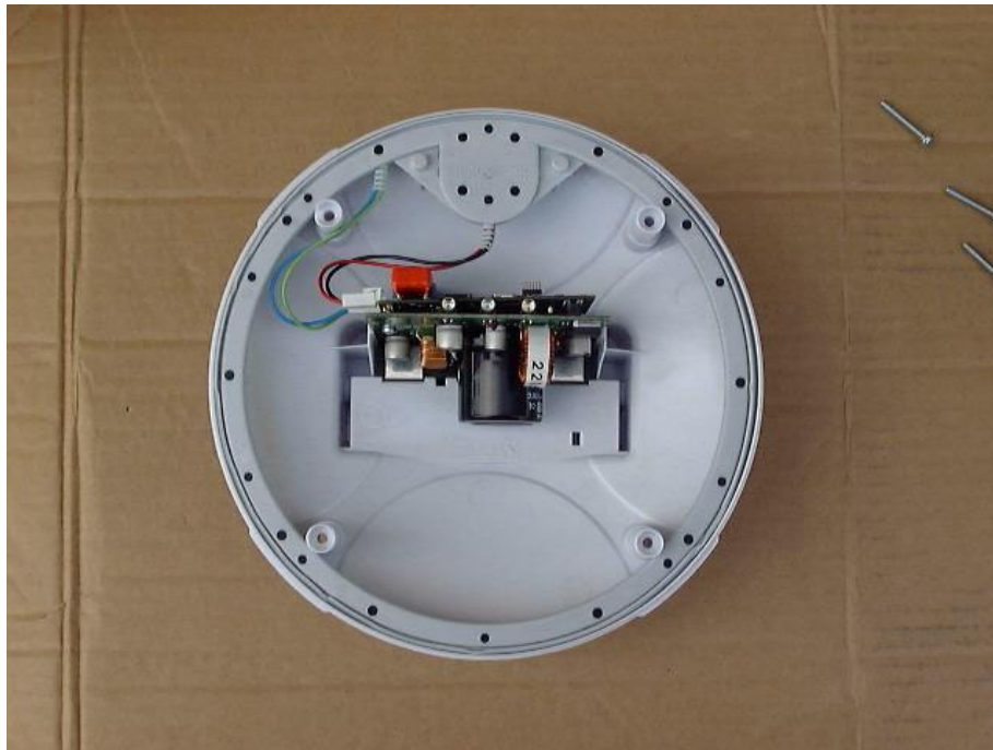
Figure 22 Rear Cover Internal View With Transmitter
