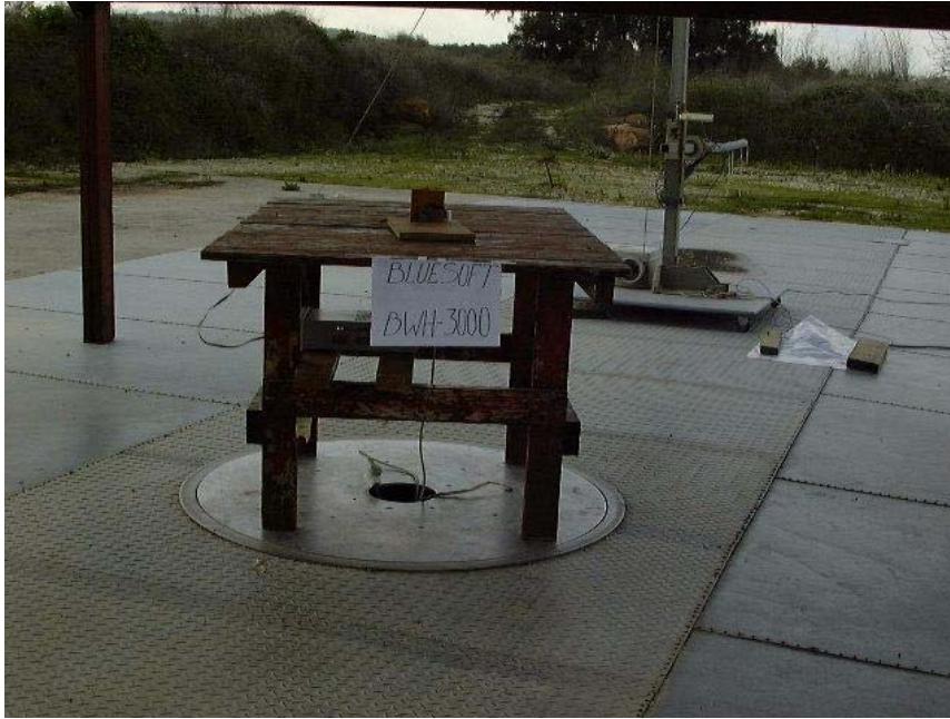
Figure 5. Spurious Radiated Emission Test Front
