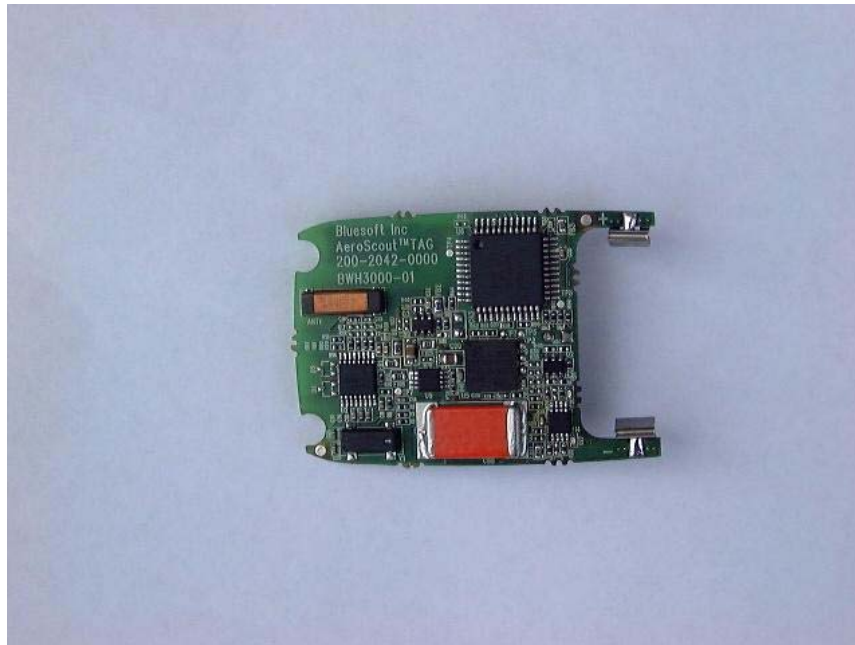
Figure 93 PCB Side 1 Without Battery
