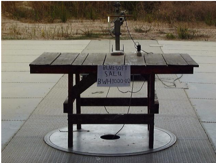
Figure 3. Spurious Radiated Emission Test Front
