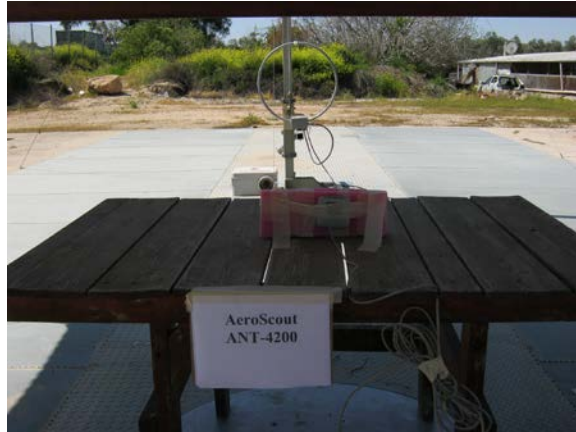
Figure 2. Radiated Emission Test 9 kHz – 30 MHz
