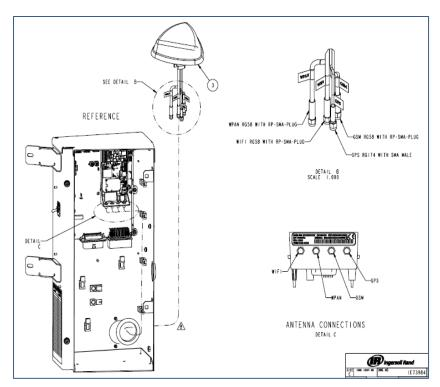
The illustration below is showing how antenna system is installed to the unit.
