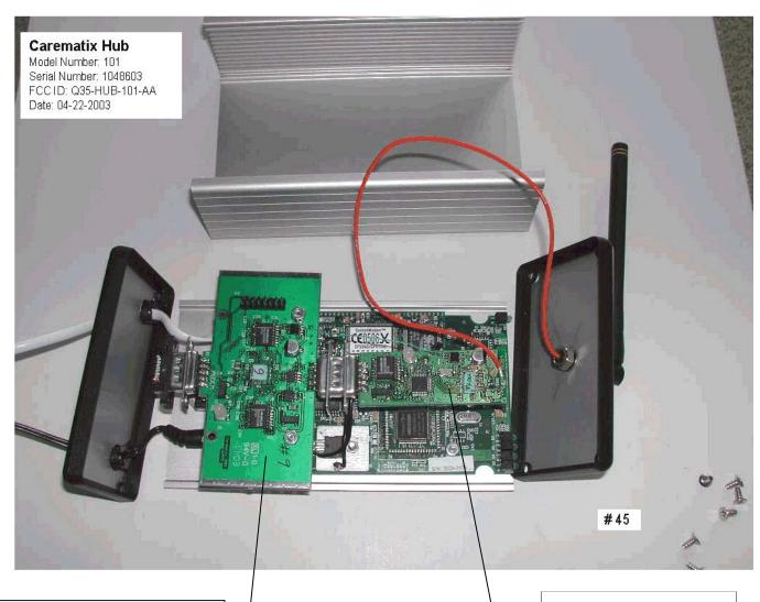
Communication Controller(KOMP) Board (Top View) Transceiver (HUB4) Board (Top View)
