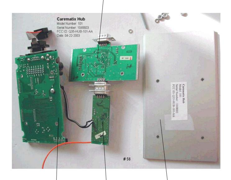
ConnectOne iModem Mother Board (Bottom View) Transceiver (HUB4) Board (Bottom View)
