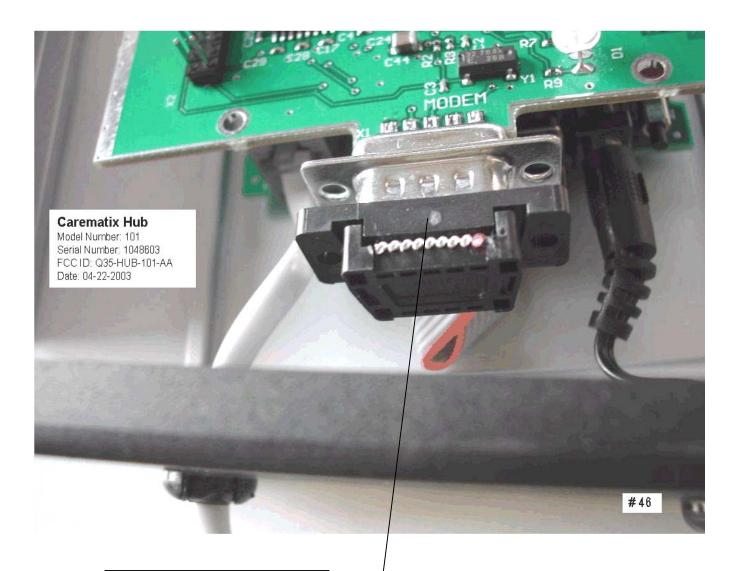
DB9 Female Ribbon Cable Connector that Connects KOMP to ConnectOne Board
