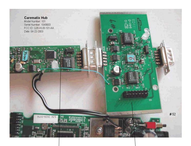
Transceiver (HUB4) Board (Top View)
