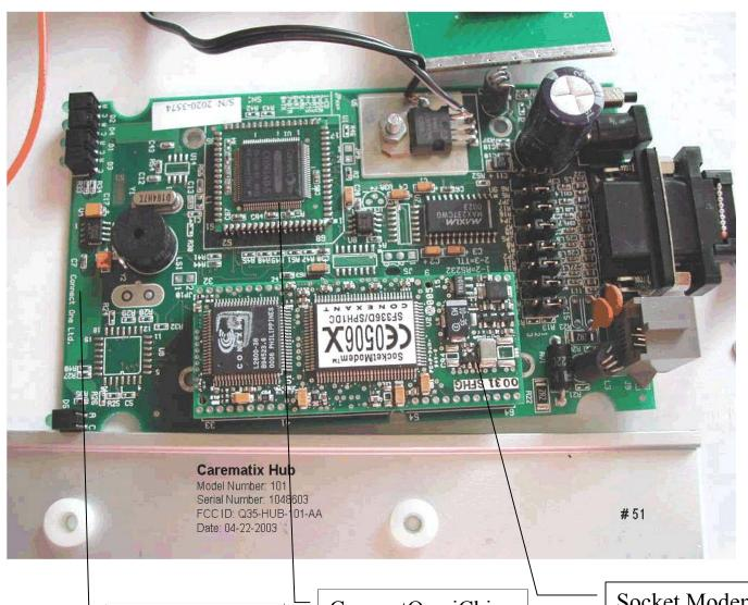
ConnectOne iModem Mother Board (Top View) ConnectOne iChip C0561AD-S (Top View) Socket Modem (Top View)
