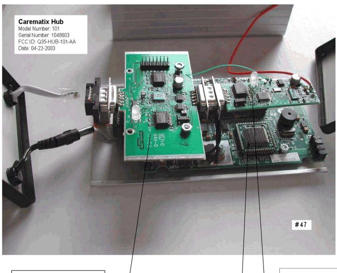
Communication Controller(KOMP) Board (Top View)
