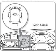
Do not install CM-HS1 on or near air conditioner duct to avoid condensation. Condensation will result in some electronic component to malfunction, damaging the unit. Also, avoid installing the unit directly in the path of front speaker of the car stereo (voice route) to minimize echo.
