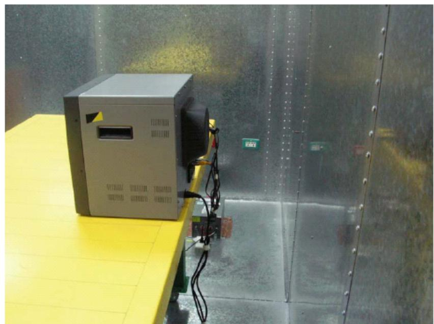
. Photographs of Radiated Emission Test Configuration
