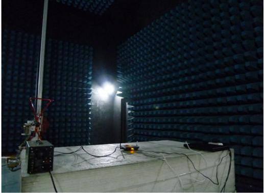
Radiated Emission Set up Photos (Above 1GHz)
