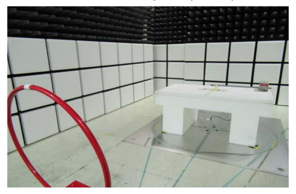
Radiated Emission Setup Photos (30MHz~1GHz)
