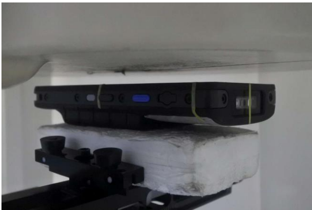
Front, Test Separation 10 mm for Battery2&3
