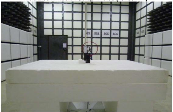
Radiated Emission Setup Photos (30MHz~1GHz)
