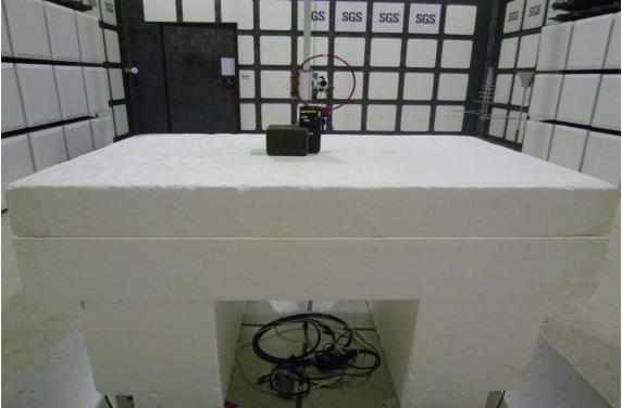
Radiated Emission Setup Photos (30MHz~1GHz)
