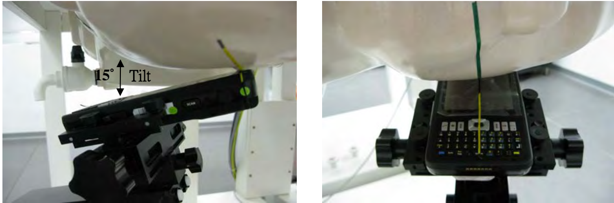
Fig.6 Left Head Section / Ear-Tilt Position(15°)
