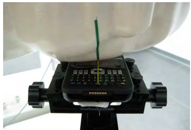
Fig.5 Left Head Section / Cheek-Touch Position
