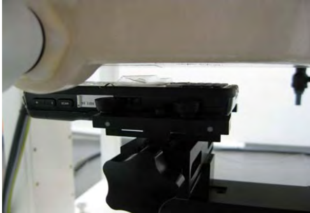
Fig.7 EUT front to flat phantom
