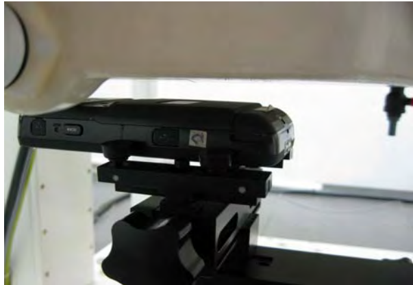
Fig.8 EUT back REID to flat phantom
