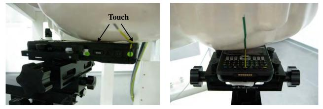
Fig.5 Left Head Section / Cheek-Touch Position
