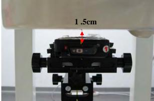
Fig.7 EUT front to flat phantom
