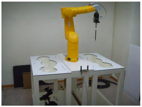
Fig.1 Photograph of the SAR measurement System
