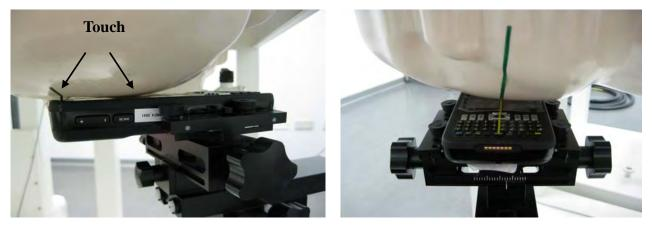
Fig.3 Right Head Section / Cheek-Touch Position
