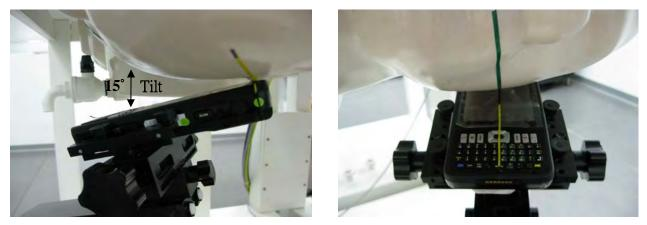
Fig.6 Left Head Section / Ear-Tilt Position(15°)
