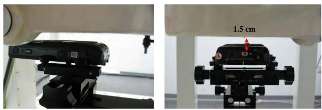
Fig.8 EUT back REID to flat phantom
