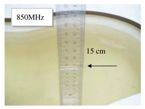
Photograph of the Tissue Simulant Fluid liquid depth 15cm
