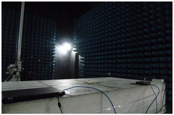
Radiated Emission Set up Photos (Below 1GHz)
