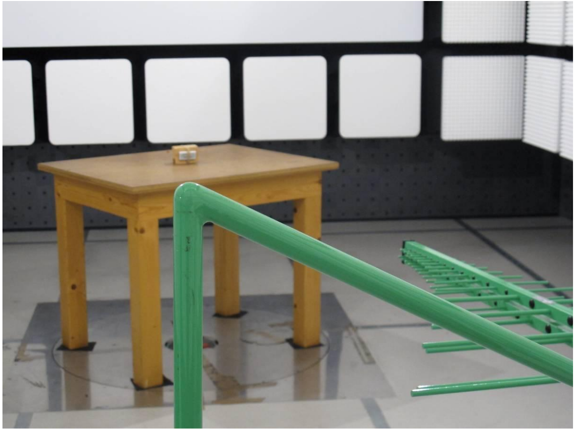
Photograph 1: Test setup radiated emissions (30 - 1000 MHz)
