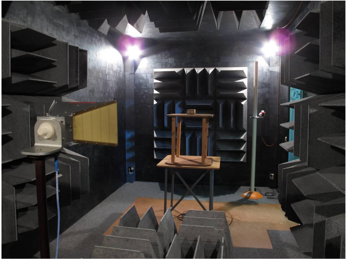
Photograph 3: Test setup radiated emissions (1 – 13 GHz)
