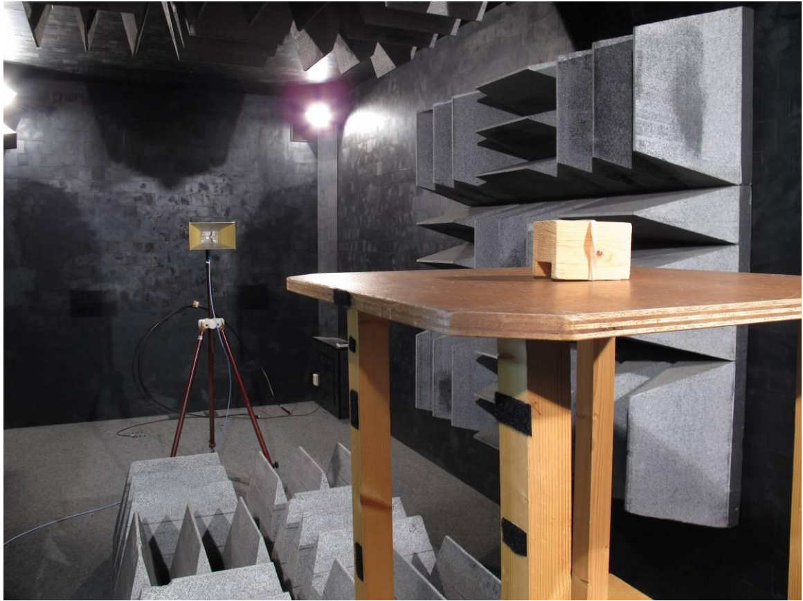
Photograph 4: Test setup radiated emissions (1 – 13 GHz)
