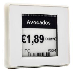
The EE-153R is a black/white/red e-paper based electronic shelf label with a screen size of 1.54" and with 802.15.4 based wireless communication.
