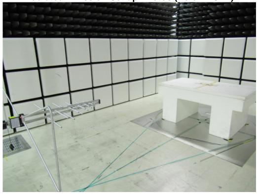
Radiated Emission Set up Photos (Above 1GHz)
