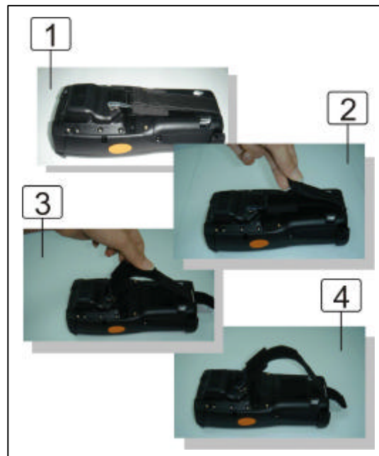
Figure 2-7 Release the Hand strap from PDT
