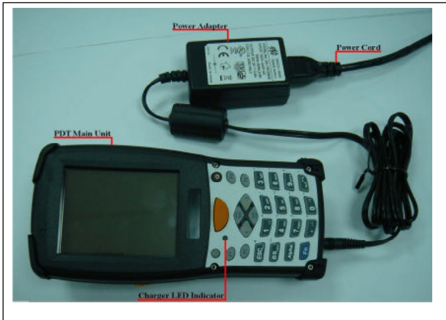
Figure 2-11 Charging with power adapter (PHL-7100 shown)
