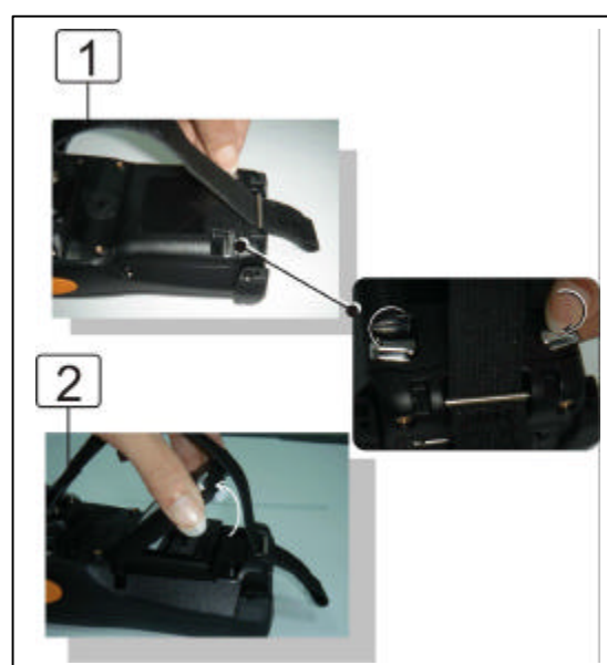
Figure 2-8 Detach the battery cover from PDT
