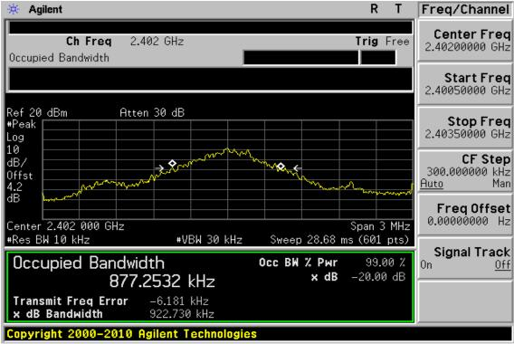
20dB Bandwidth Test Data CH-Mid
