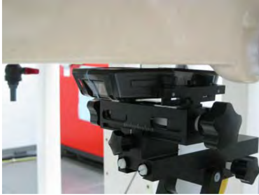
Fig.3 EUT front side to flat phantom
