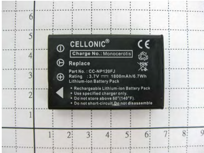
Fig.8 Back view of battery
