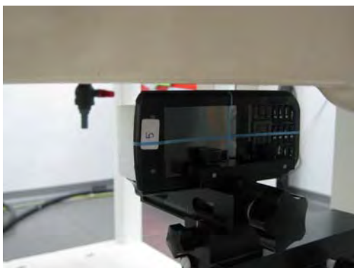
Fig.5 EUT Left side to flat phantom
