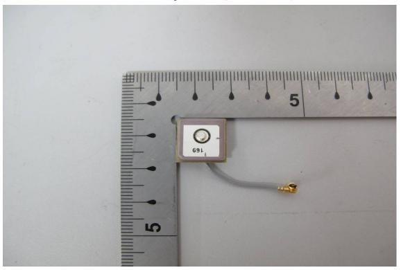
Internal View of EUT - 9 (GSM Antenna)
