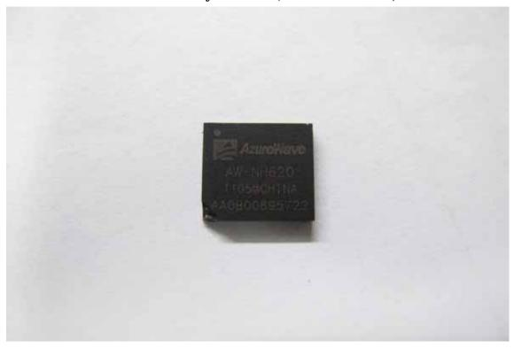
Internal View of EUT – 11 (WLAN/BT Module)
