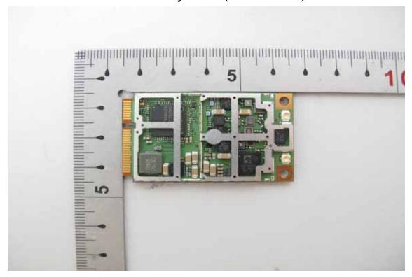
Internal View of EUT – 7(WWAN module)
