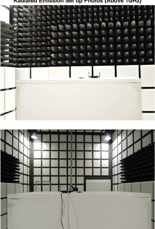
Radiated Emission Set up Photos (Above 1GHz)
