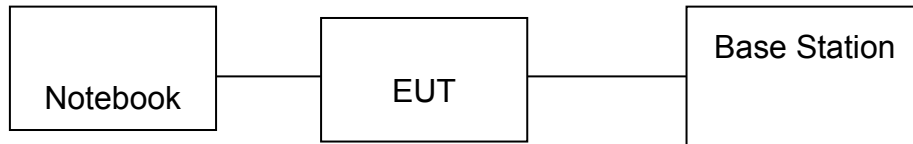
Fig. 2-2 Conducted (Antenna Port) Configuration
