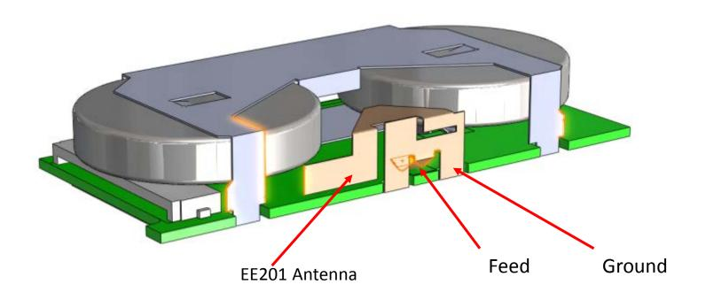
EE201 antenna is a sheet metal PIFA with -4dBi Gain
