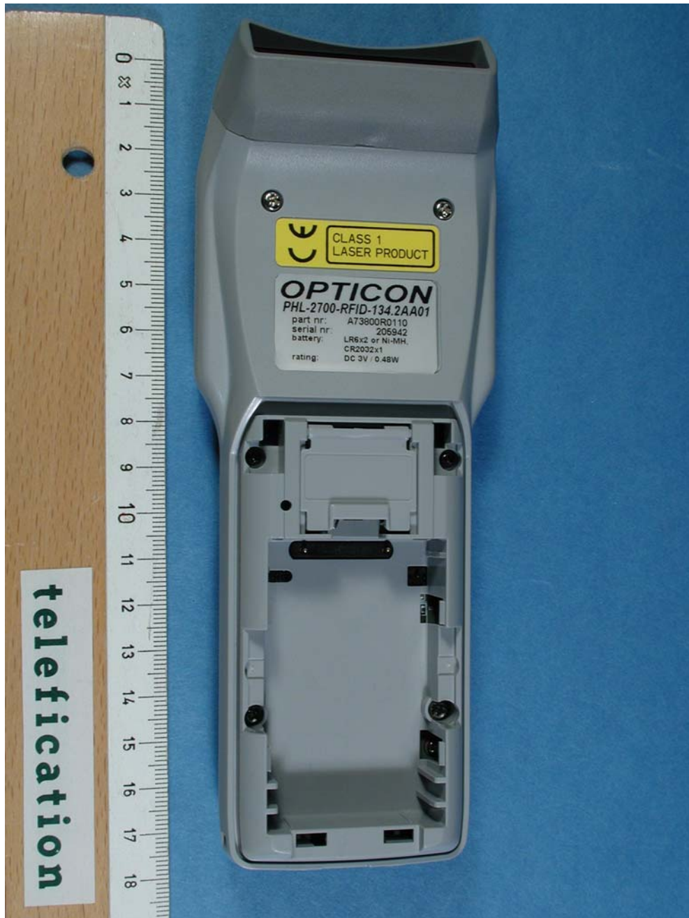
Rear view of equipment with battery and battery cover removed
