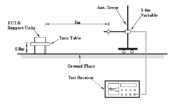
The deactivation test was performed in the 3 meters chamber test site, using the setup accordance with the ANSI C63.4 - 2009. The specification used was the FCC 15.231(a) limits.
