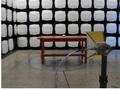
Measurement of Radiated Emission Test 1GHz-5GHz
