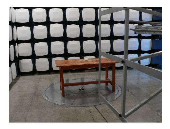
Measurement of Radiated Emission Test
