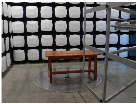
Measurement of Radiated Emission Test
