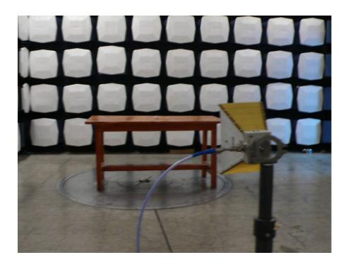
Measurement of Radiated Emission Test 1GHz-5GHz
