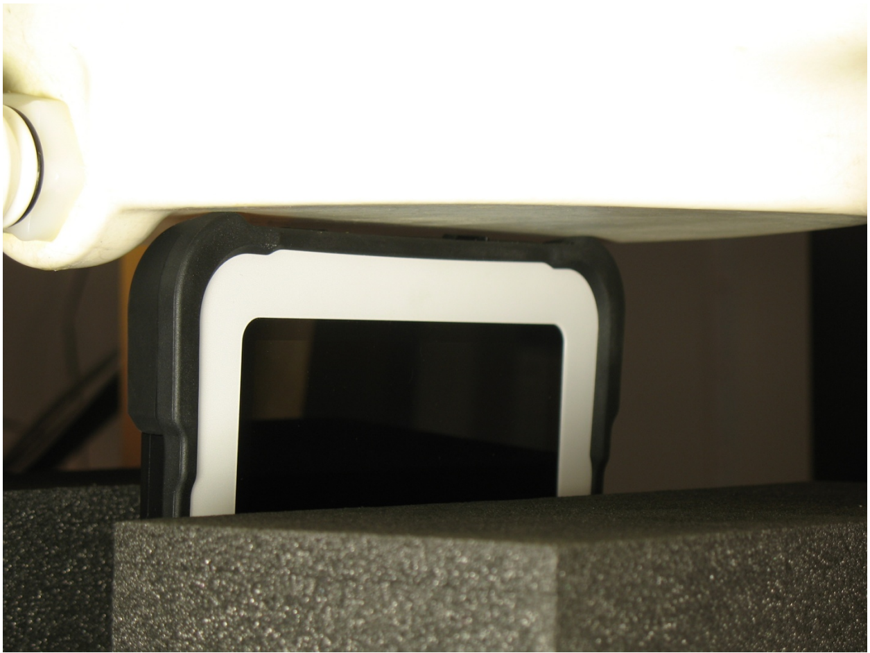
Figure 3: Device Positioning for SAR Scans – Side Edge Nearest WLAN Antennas
