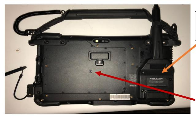
RFID Module attached to Host
