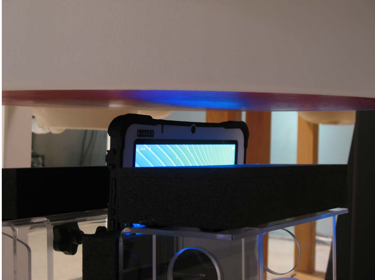
Figure 17: Device Positioning for SAR Scans – Lap Position – Back Against Phantom with 15mm Spacing
