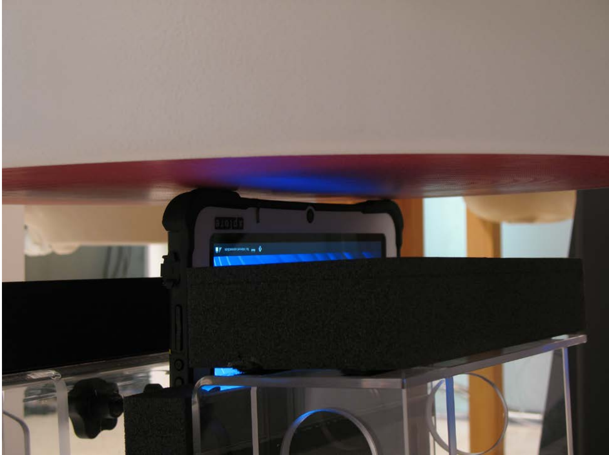
Figure 16: Device Positioning for SAR Scans – Lap Position – Back Against Phantom with no Spacing
