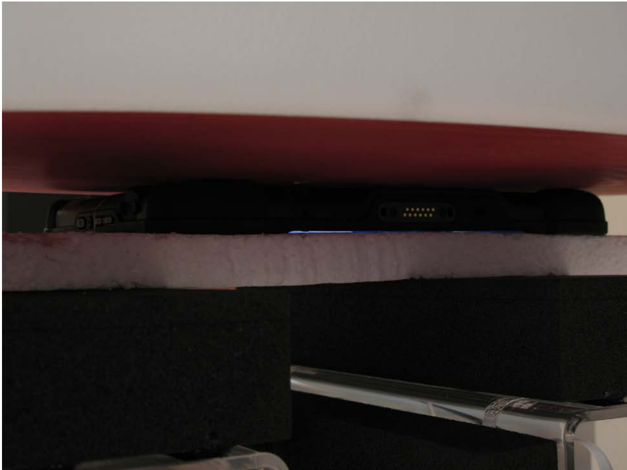
Figure 14: Device Positioning for SAR Scans – Lap Position – Back Against Phantom with No Spacing
