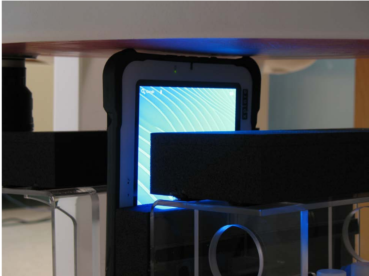
Figure 18: Device Positioning for SAR Scans – Side Edge Nearest WWAN Antennas with no Spacing
