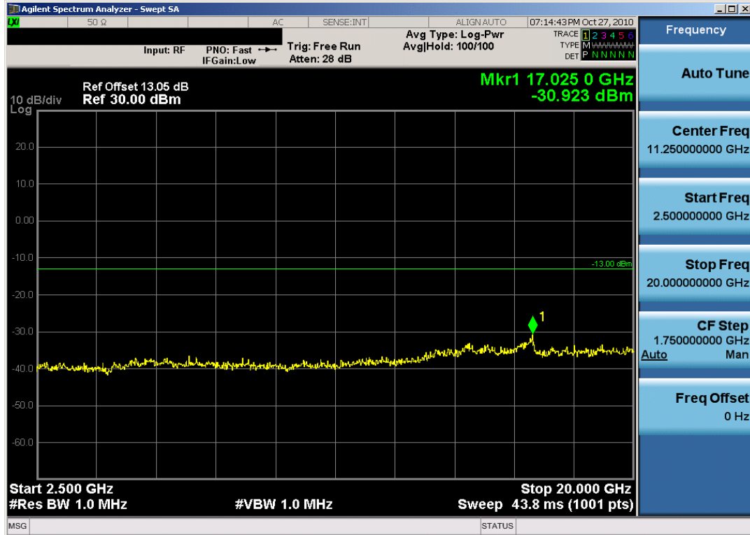
Plot 7-19. Conducted Spurious Plot (PCS GSM Mode – Ch. 810)
