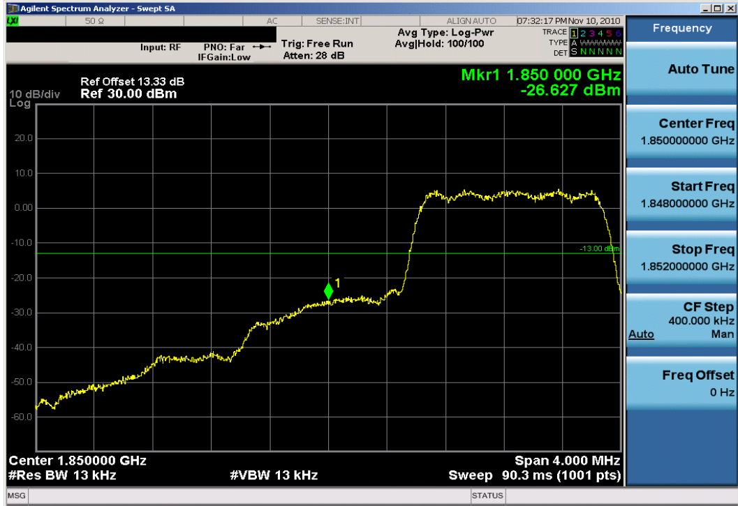
Plot 7-59. Band Edge Plot (PCS CDMA Mode – Ch. 25)
