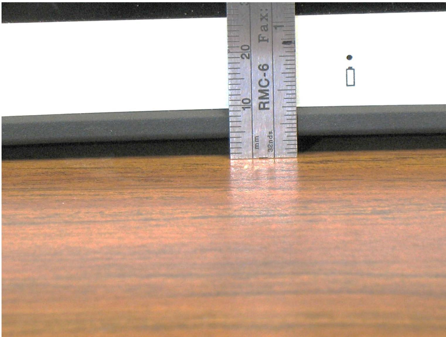
Distance From Right Edge to Flat Surface (Measured with Gauge Block – 3.2mm)
