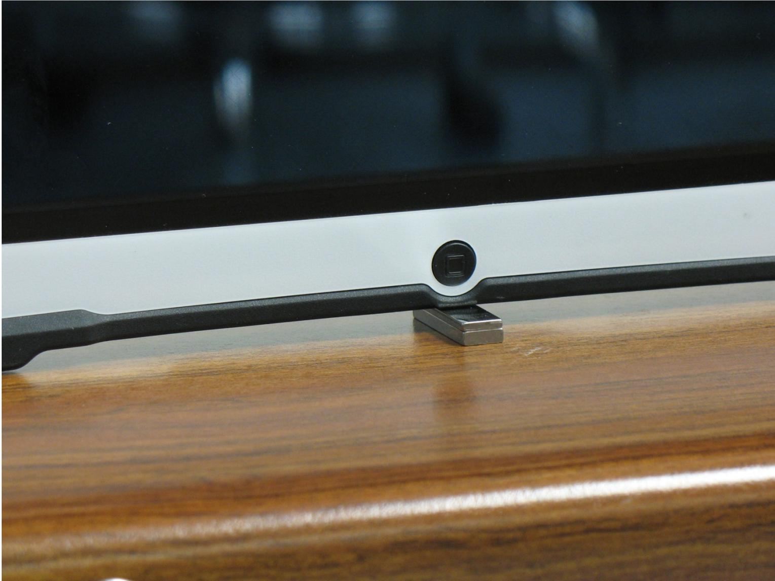
Distance From Bottom Edge to Flat Surface at location of WWAN Antenna (antenna edge closest center of tablet) (Measured with Gauge Block – 4.7mm)
