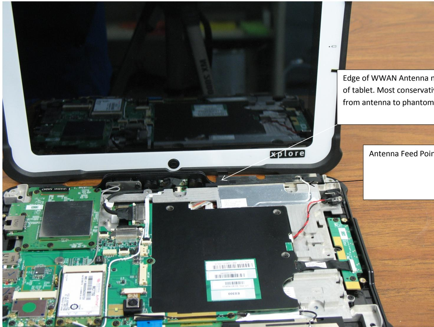
Edge of WWAN Antenna nearest center of tablet. Most conservative distance from antenna to phantom.
