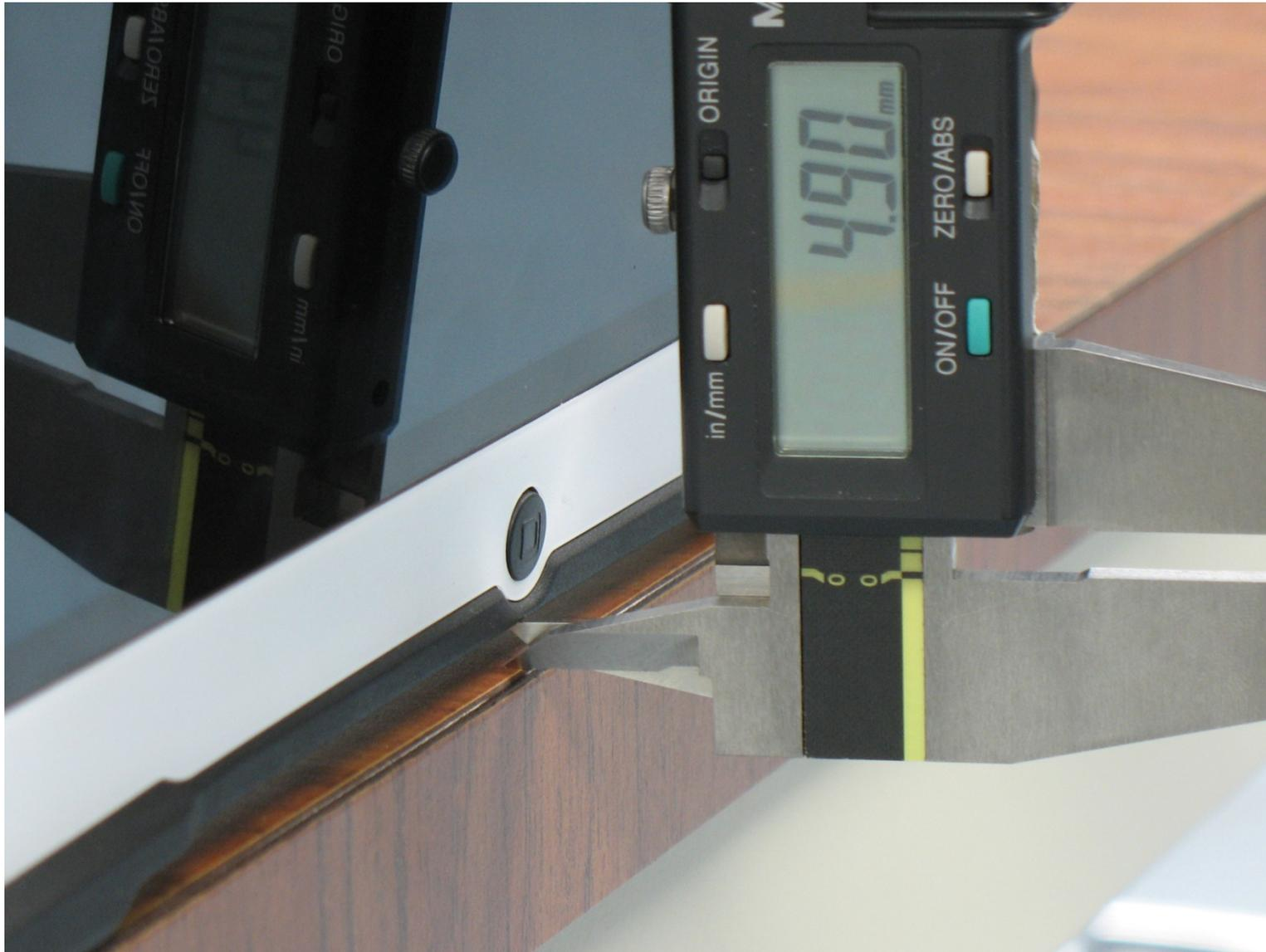
Distance From Bottom Center to Flat Surface (Measured with Gauge Block – 4.9mm)
