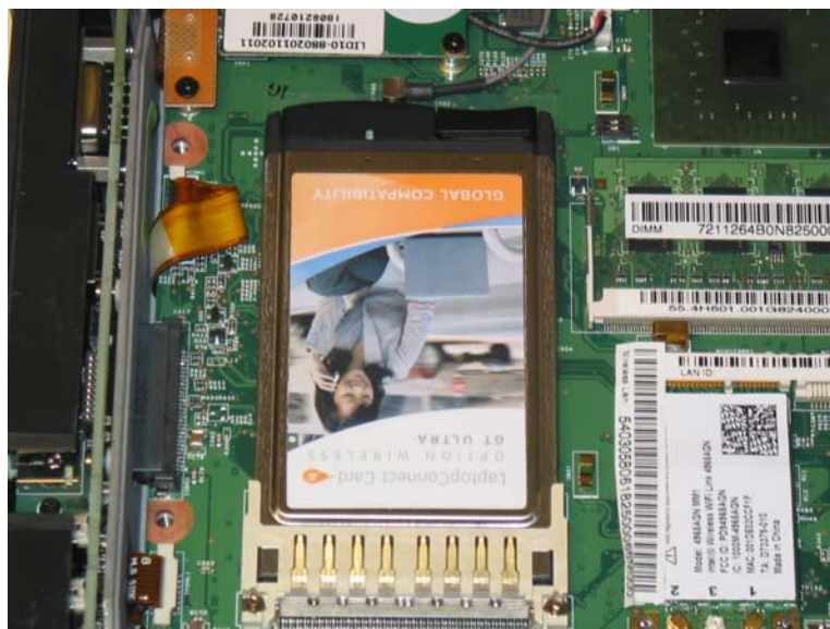
WWAN Module Installed
