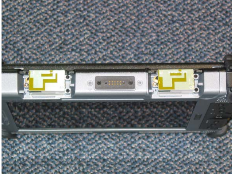
View of Both Antennas
