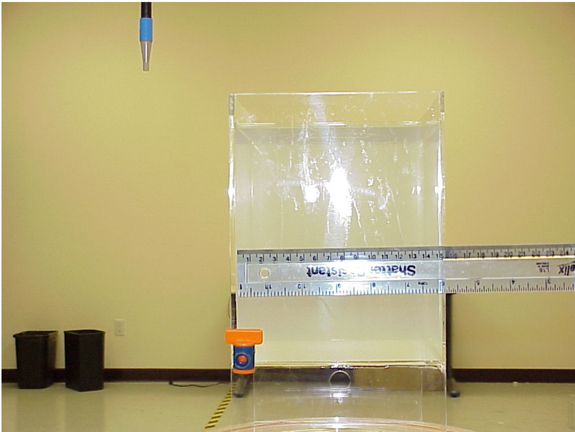
Photo 4. Photo to demonstrate 15 cm Z-axis flat phantom
