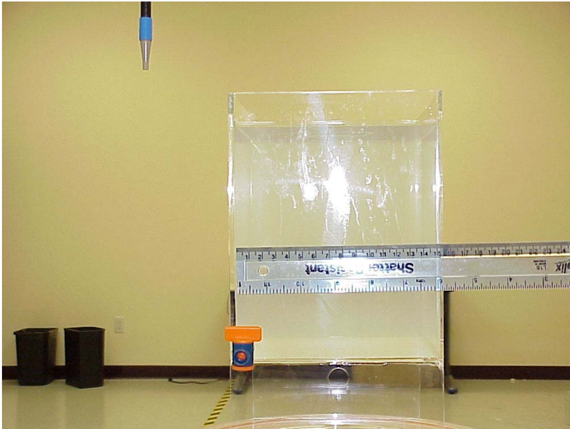
Photo 5 Photo to demonstrate 15 cm Z-axis flat phantom
