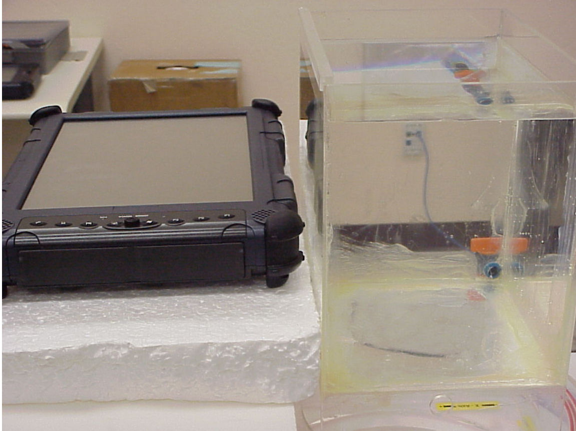
Photo 7. 2450 MHz antenna bystander position
